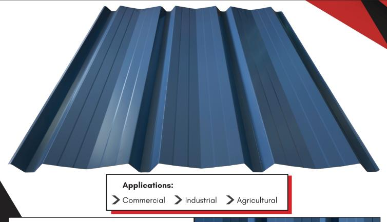
Our PBA panel is a wall panel that is highly durable and versatile. Perfect for many projects such as warehouses, storage units, and other vertical applications. This product is available in 24 and 26 gauge and can be utilized over open structual framing or solid substrate. The PBA panel has a 36" coverage with exposed fasteners. Available in 18 Sherwin Williams colors.
